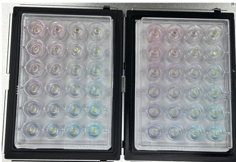
Fig. 4. Proof of concept sitting drop plates with food coloring. The OT-2 prepared a sitting drop plate with dyes to visualize correct mixing (left) compared to an experimentalist's sitting drop plate with dyes (right). A blue gradient increases from left to right, and a red gradient increases from top to bottom. Each reservoir mixture was then mixed with a yellow dye stock to mimic combining each reservoir solution with purified protein in a sitting drop.
